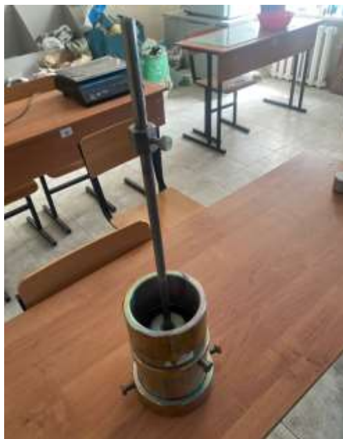
Figure 1. Standard Proctor-type compaction apparatus [Own material]
