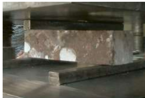
Figure 5. Photo – 2016. Testing of beam samples made from cuttings of the bottom layer of cinder concrete pavement for bending strength (the structure of the beam is non-uniform - the filler is a local gravel-sand mixture) [own material]
