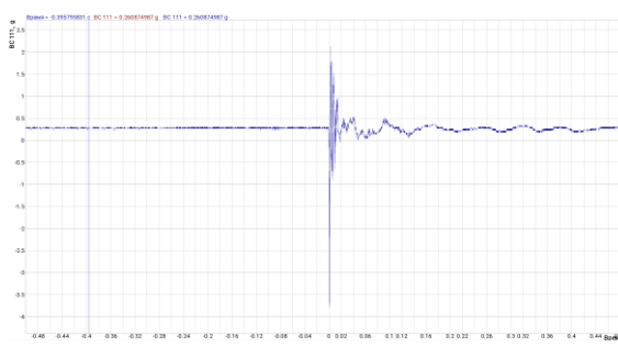
Figure 6. Accelerogram of soil-rubber mixture. Experiment 1
