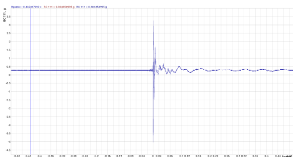
Figure 7. Accelerogram of soil-rubber mixture. Experiment 2
