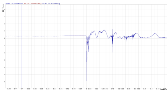
Figure 3. Accelerogram of natural soil without additives. Experiment 1
